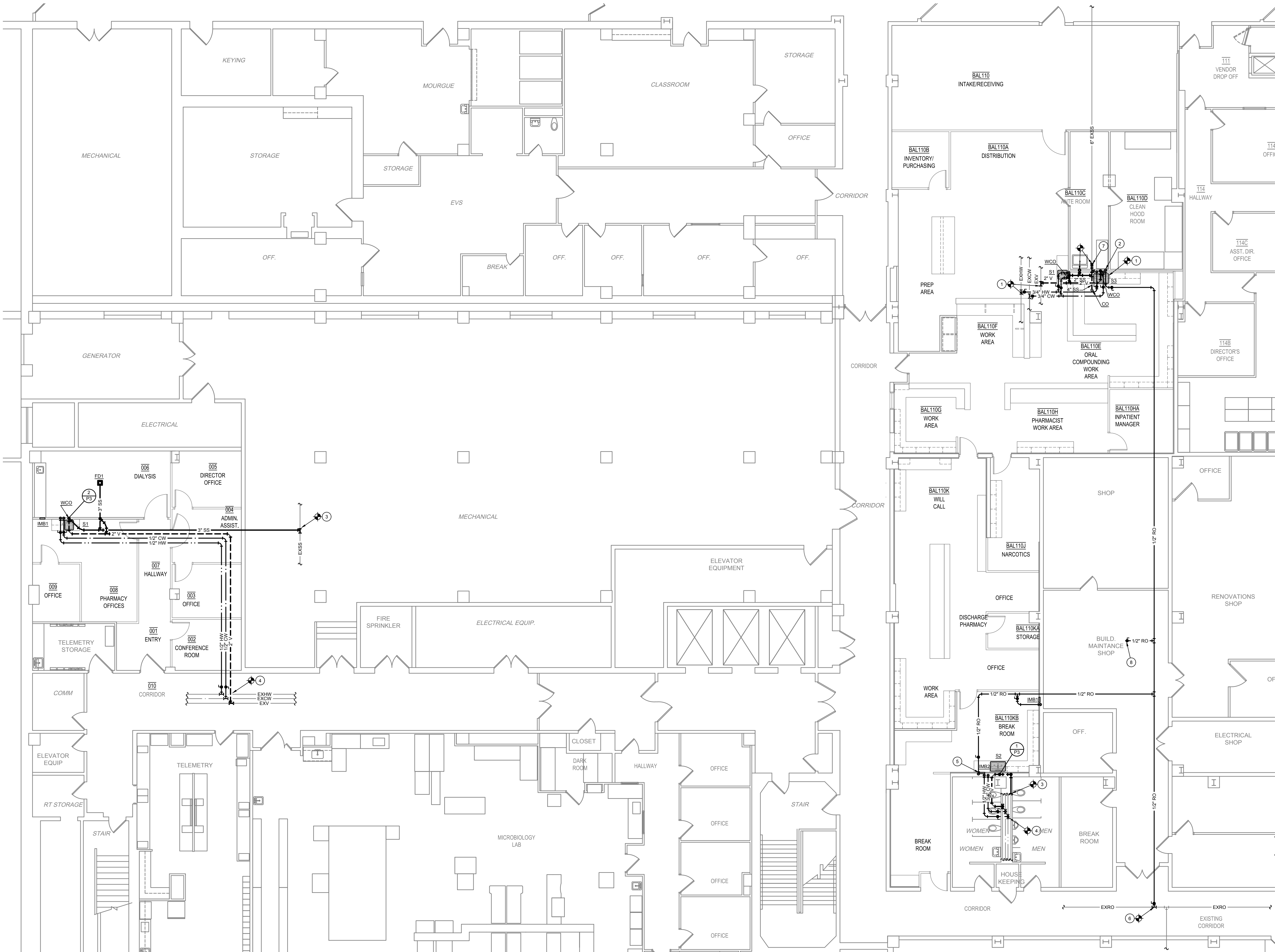
1/P2 BASEMENT PLAN - PLUMBING SEWER, WASTE, & VENT SCALE: 1/8" = 1'-0"
