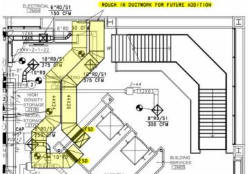
A 2HR separating wall needs to be installed at the backside of the elevators separating the ductwork shaft and elevator shaft. This wall will extend the entire length of the shaft and be included in Alternate 04.
